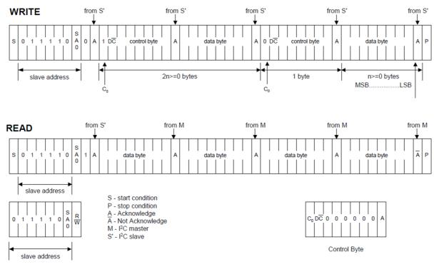
(a)I2C address bit (SA0) The slave address is following the start condition for recognition use. Two 7-bit slave addresses are "b0111100" or "b0111101" by changing the SA0 to LOW or HIGH (A0 pin acts as SA0).
