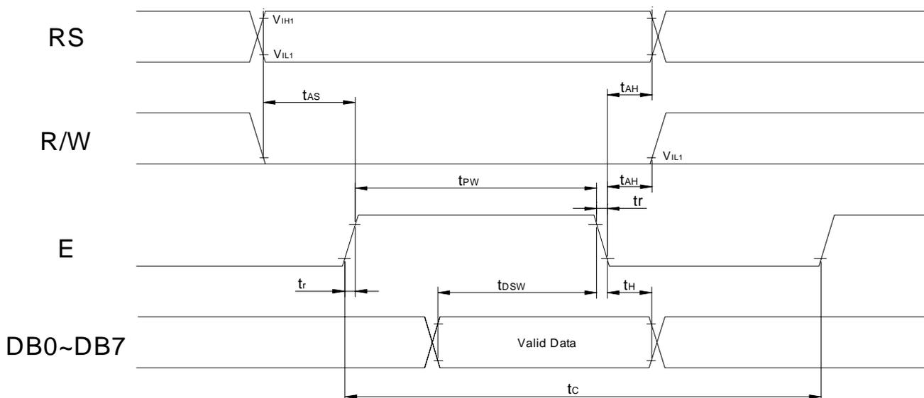
9-2-2 Read mode (reading data from module to MPU)
