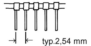
Ø hole in PCB typ. 1,0 mm
