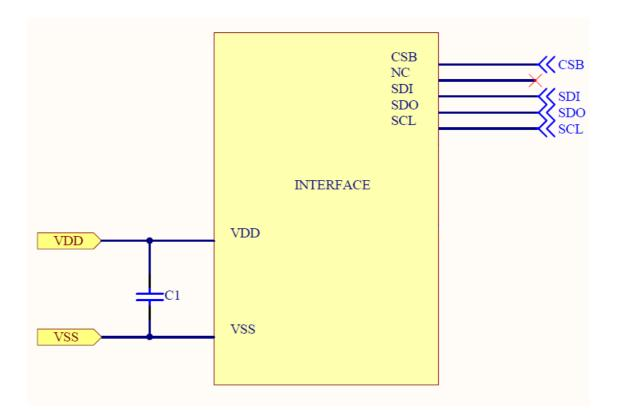
Pin connected to MCU interface: CSB,SDI,SDO,SCL C1 : 1.0uF
