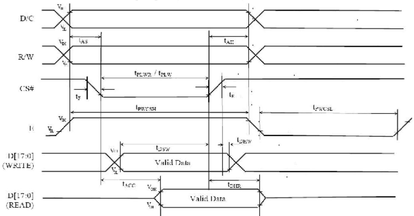
Parallel 6800-Series Interface Timing Characteristics (Use E as clock)
