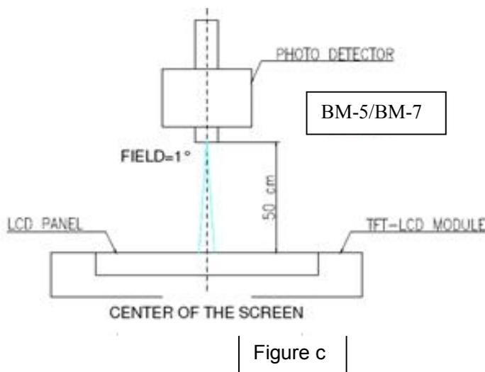
FIG.3. The definition of viewing angle
